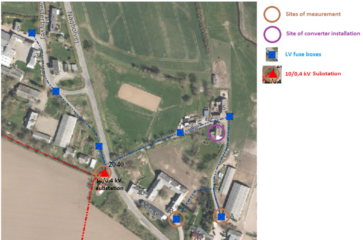
Figure 14. Aerial view of TREFOR demonstration site, with site of converter and sites of measurements shown.
